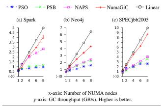
Figure 7. Scalability for three applications with large heap
