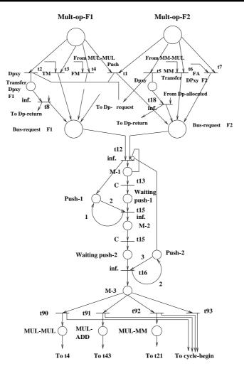
Figure 17: A pipe-lined multiplier model
