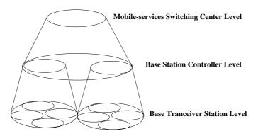
Figure 19: Physical Aggregation - GSM system
