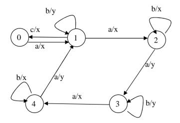
We consider an FSM with '0' as the initial state, the input set = $\{a,b,c\}$  and output set= $\{x,y\}$ .
