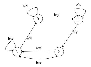
We consider an FSM with '0' as the initial state, the input set = $\{a,b\}$  and output set= $\{x,y\}$ .
