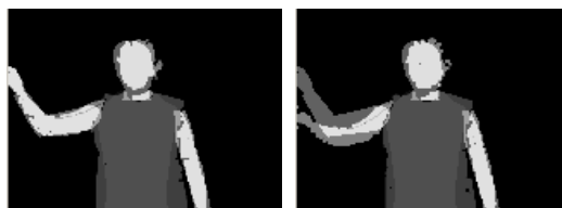
Figure 3. Superposition of the 3D model registered at time t with the segmented video images at t and t+1 .
