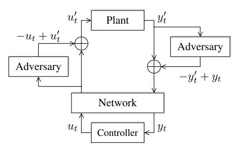
Figure 1: Representation of a cyber-physical industrial attack against a networked control system.  $u_t$  and  $y_t$  represent the correct input and output vectors of the system.  $u'_t$  and  $y'_t$  represent the attack vectors.
