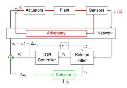
Figure 2: Signature-based protection in cyber-physical systems [24].
