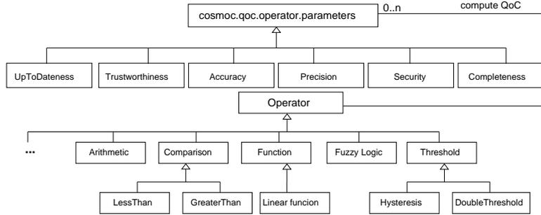
Fig. 5: Relation between QoC Parameters and COSMOS Operators
