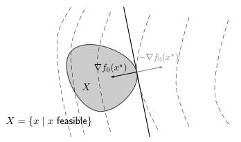
Equivalent condition:  $-\nabla f_0(x^*) \in \mathcal{N}_X(x^*)$  (normal cone)
