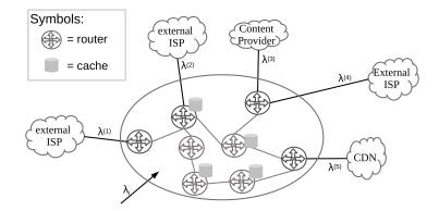
Figure 3.1: Model of the ISP. The ISP is connected to third party networks through external links  $l_1, l_2, \ldots, l_5$ .
