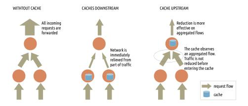
Figure 2.2: Flow reduction and aggregation.
