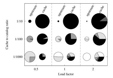
Figure 5.5: Single-AS scenario: Contributions of cache and upstream links. Circle size reflects relative cache vs upstream contribution, and the breakdown reports the qualities of both contributions.
