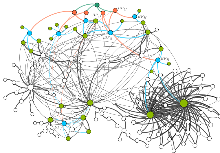
Fig. 4 Mission dependency model and resource dependency model obtained and learned from data of the use case partner. BF_R represents a business function (blue) subject to handling remote terminal units (RTUs), which are visible as the lower right clouds of nodes, where the central nodes are business critical devices (green). Business processes shown in orange, business company in dark green. Thicker and darker edges represent higher dependency degrees. Visualized using Gephi [50]
